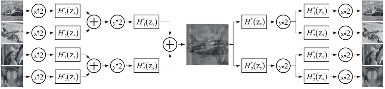
Fig. 1. Scheme of 4-channel image transmultiplexer
