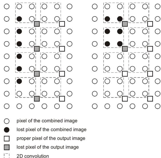
Fig. 2 Scheme of lost pixels, 6 pixels per packet and  $K = 2$ .
